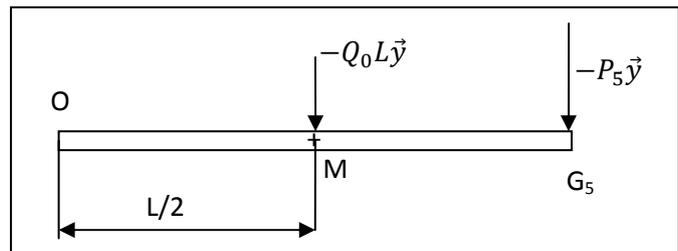
$$\text{Donc} \quad \{\text{Bâti} \rightarrow \text{Poutre}\}_O = \left\{ \begin{array}{c} (Q_0L + P_5)\vec{y} \\ (Q_0\frac{L^2}{2} + P_5L)\vec{z} \end{array} \right\}_O$$
